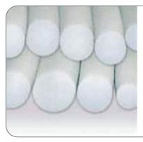
Dynaflex round polyethylene profiles is used to fill up expansions joints, gaps of sides of the windows and doors etc. It is produced from the diameter of 8 mm up to 100 mm. It minimizes the consumption of the filling material such as acrylic or polyurethane. I absorbs the thermal tensions and building movements.
